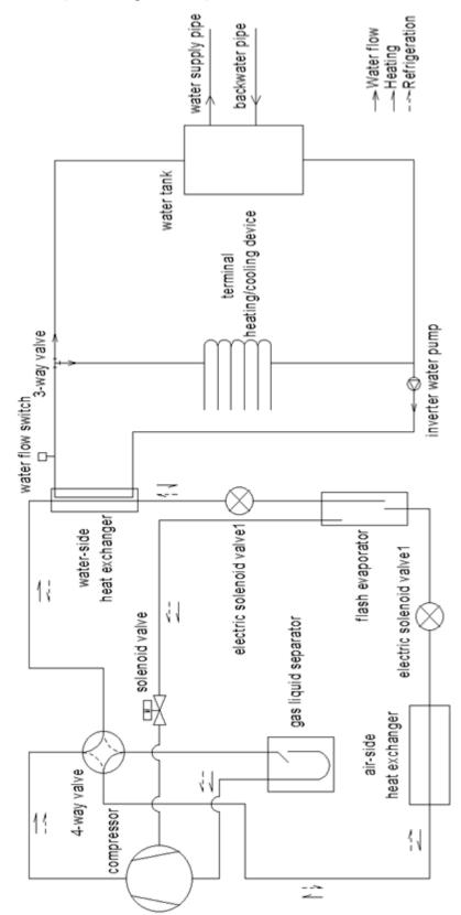
NOTE: In actual engineering, terminals heating/cooling device are selected by the user.
