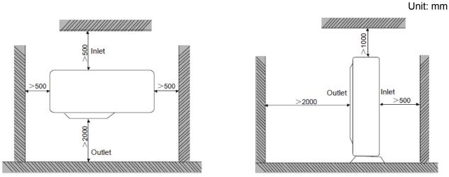
**NOTE:** In confederation of space restriction, for the left-handed figure, except the outlet side, distance between the unit and the nearest barrier at other three sides are allowed to be no less than 500mm; for the right-handed figure, distance between the inlet side and the nearest barrier is allowed to be no less than 500mm.
