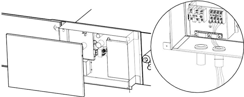
Figure 3-4 Diagram of electric box wiring
