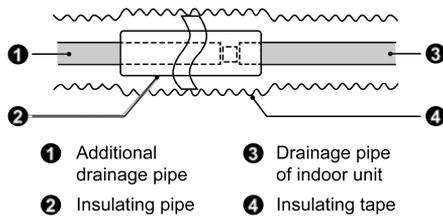
Figure 3-8 Thermal insulation of drain pipes
