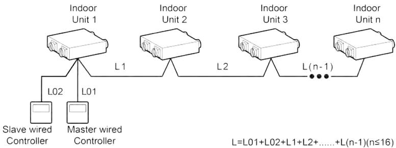
Figure 3-2 Diagram of wired controller control connection
