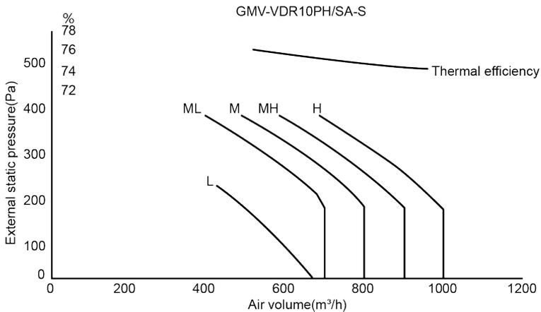
Figure 3-13 The flow/pressure diagram
