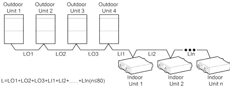
Figure 3-3 Diagram of IDU and ODU control connection
