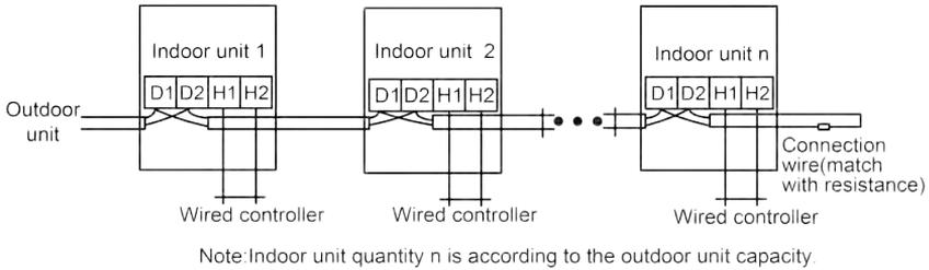
Figure 3-6 Diagram 2 of wiring board
