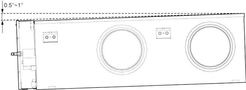
Figure 3-12 Inclination of the unit
