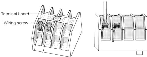
Figure 3-5 Diagram 1 of wiring board
