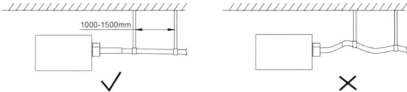
10) Make sure the weight of drain pipes won't be borne by the unit.
