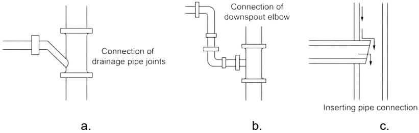
9) Keep the drain pipe downward with an inclination of  $1^{\circ} \sim 2^{\circ}$  or more.
