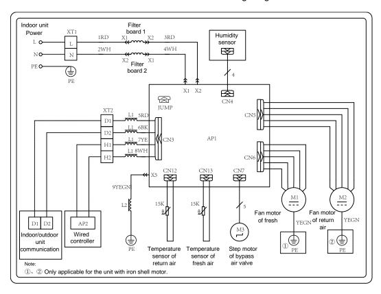
FHBQGL-D5DA-T Internal Wiring Diagram
