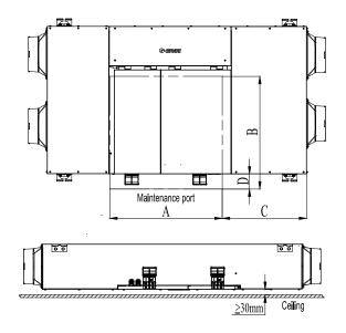
Fig. 9 Diagram of Maintenance Port
