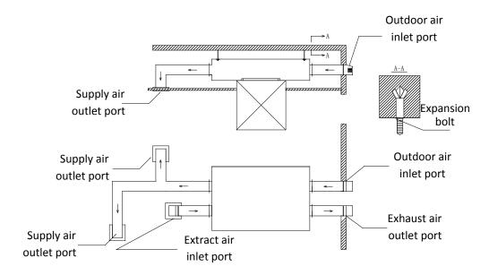
Fig. 8 Installation Diagram
