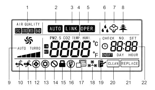
Fig. 4 LCD Graphics of Wired Controller
