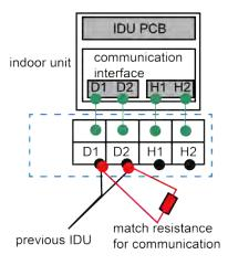
Fig. 14 Wiring Board
