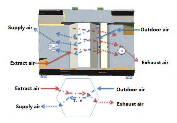
Fig. 1 Operation Principle Diagram of this unit
