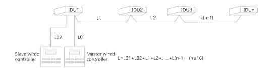
Fig. 16 Wiring Diagram of Wired Controller
