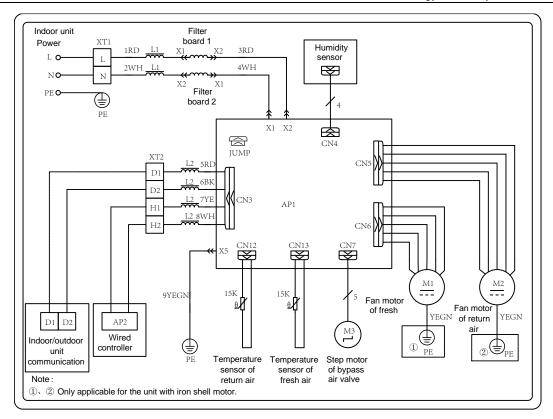
FHBQGL-D3.5DA-T Internal Wiring Diagram
