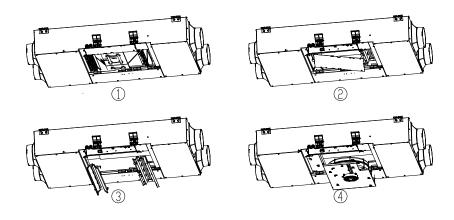
Fig. 19 Disassembly Diagram of Component
