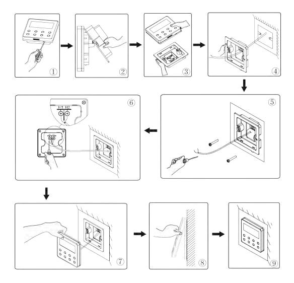
Fig. 17 Installation Diagram for Wired Controller
