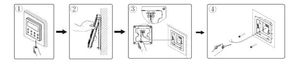
Fig. 18 Disassembly Diagram of Wired Controller
