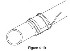
6) Wrap the temperature sensor with insulator.
