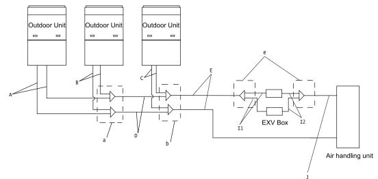
Figure 3-5 Several AHU-KITs to one AHU
