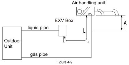
When several AHU-KITs are connected to one AHU, the piping installation diagram is as follows:
