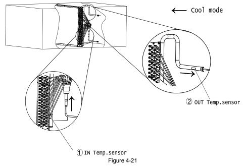
①IN Temp. sensor (Liquid Temp. sensor)
