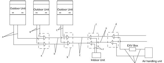
Figure 3-4 One AHU-KIT to one AHU
