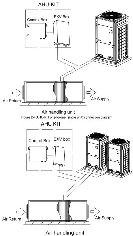
Figure 2-5 AHU-KIT one-to-one (combination outdoor unit) connection diagram
