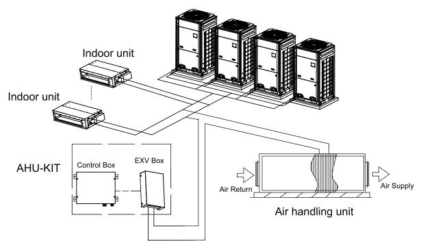
Figure 2-6 AHU-KIT one-to-more (hybrid connection) connection diagram
