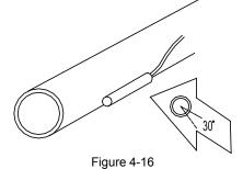
3) Fix the temperature sensor with insulating aluminum tape in order to ensure good heat transference.
