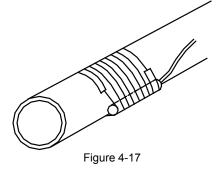
4) Cover the temperature sensor with rubber belt to prevent looseness of temperature sensor.
