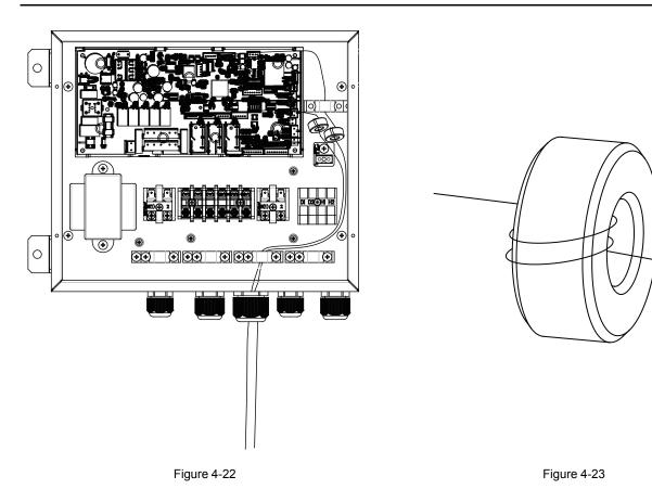
The quantity of expansion valve coil is determined by the actual number of fittings, The length of EXV Cable wire is 10 m (71,140,280,560 type) or 2.5 m (36 type).
