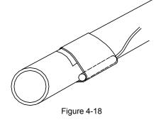
5) Use two wire ties to bind the temperature sensor securely.
