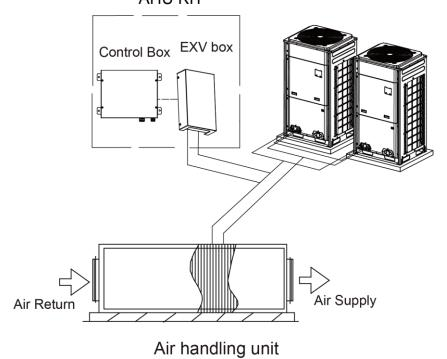
Fig.2.5.2 AHU-KIT one-to-one (combination outdoor unit) connection diagram
