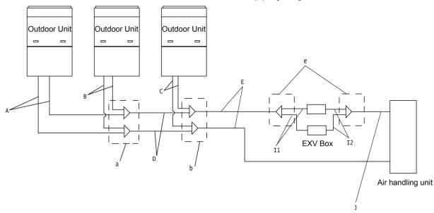
Fig.3.5.2 Several AHU-KITs to one AHU
