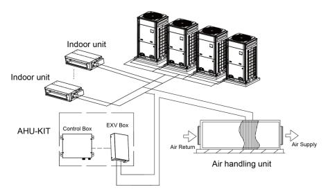
Fig.2.5.3 AHU-KIT one-to-more (hybrid connection) connection diagram
