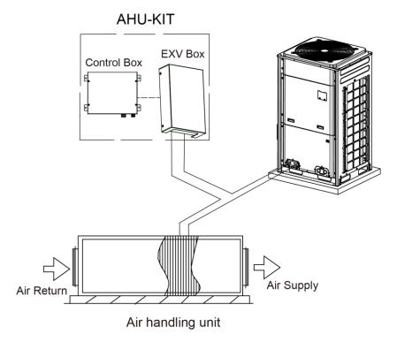
Fig.2.5.1 AHU-KIT one-to-one (single unit) connection diagram AHU KIT
