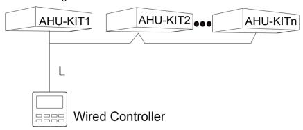
Fig.3.3.2 One wired controller to several AHU-KITs
