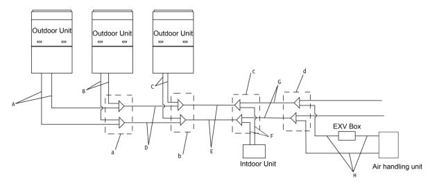
Fig.3.5.1 One AHU-KIT to one AHU
