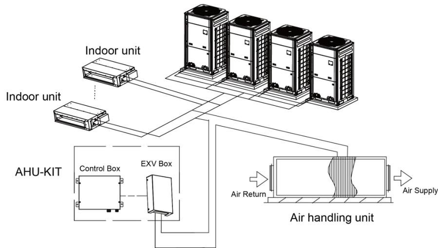
Fig.2.5.3 AHU-KIT one-to-more (hybrid connection) connection diagram
