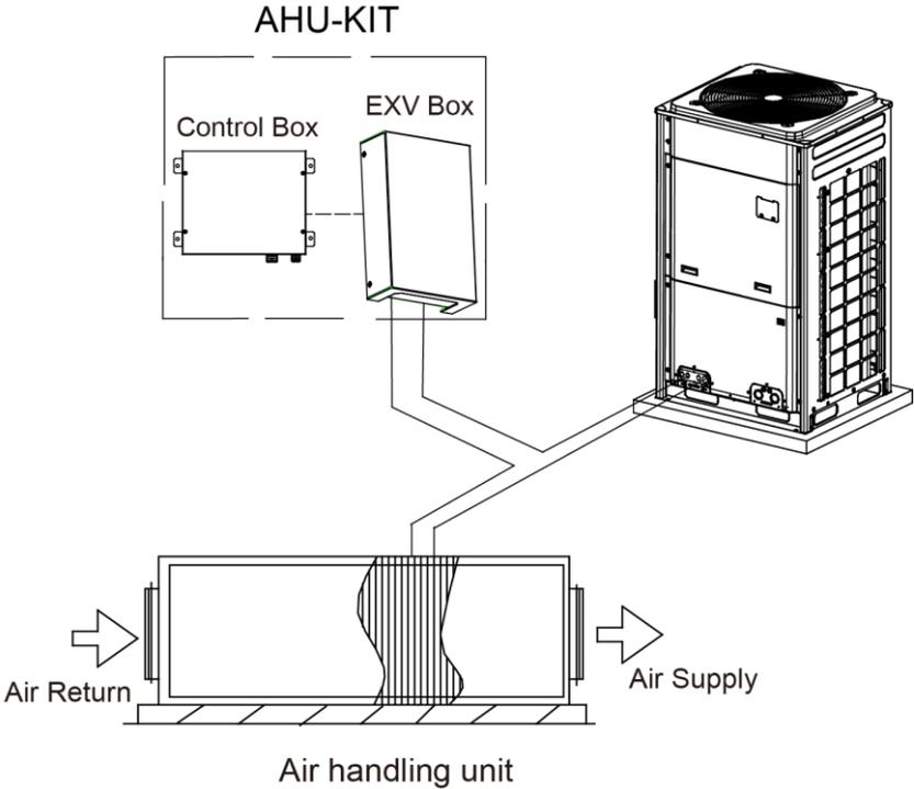
Fig.2.5.1 AHU-KIT one-to-one (single unit) connection diagram
