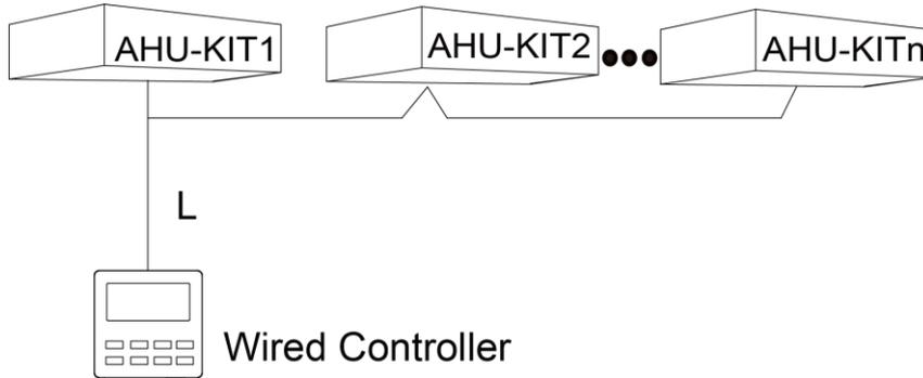
Fig.3.3.2 One wired controller to several AHU-KITs
