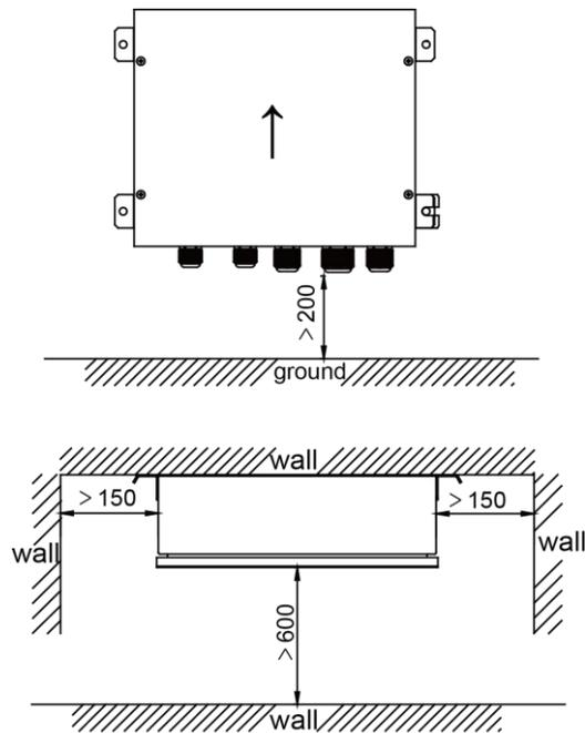
The control box must be installed upwards as the direction of the arrow shown in the figure
