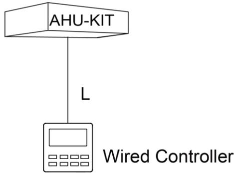
Fig.3.3.1 One wired controller to one AHU-KIT
