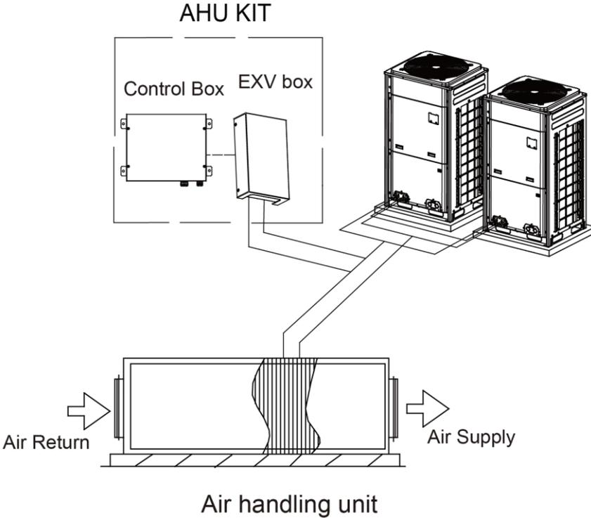
Fig.2.5.2 AHU-KIT one-to-one (combination outdoor unit) connection diagram
