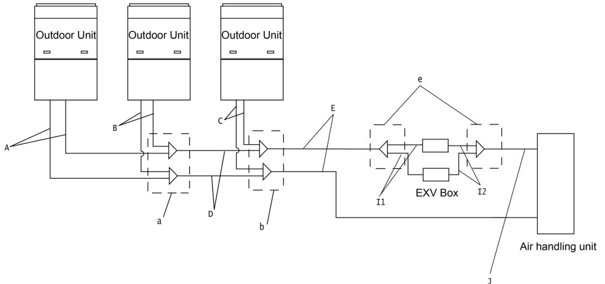
Fig.3.5.2 Several AHU-KITs to one AHU
