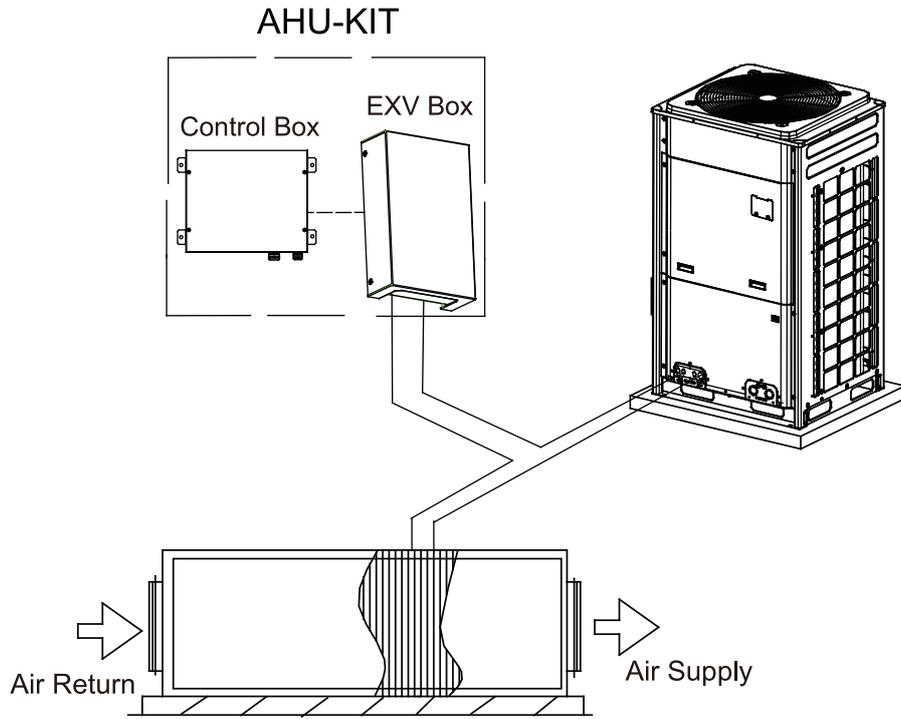
Figure 2-4 AHU-KIT one-to-one (single unit) connection diagram
