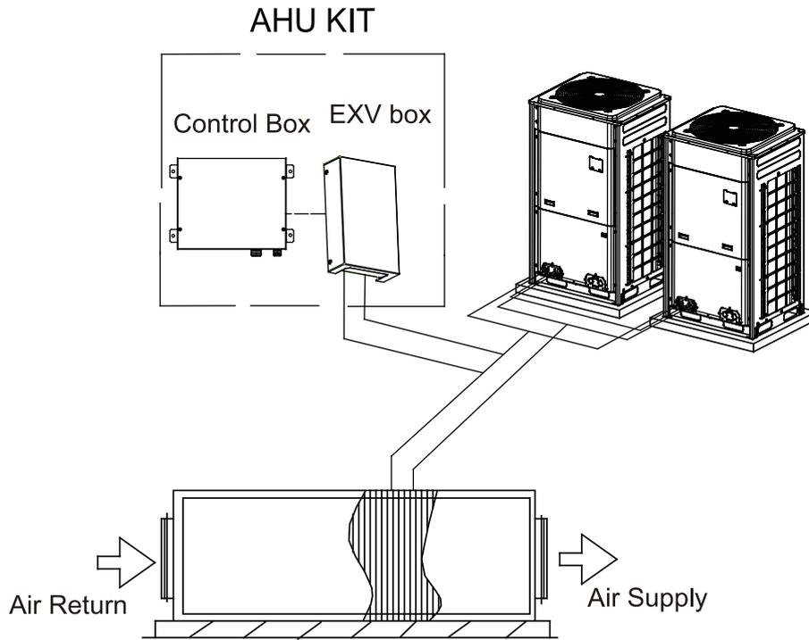
Figure 2-5 AHU-KIT one-to-one (combination outdoor unit) connection diagram
