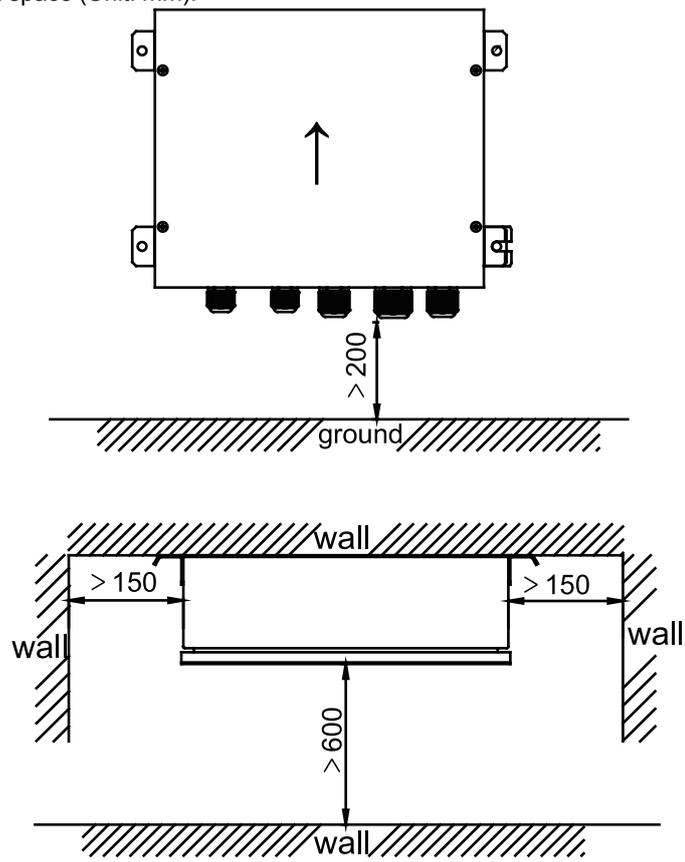
The control box must be installed upwards as the direction of the arrow shown in the figure
