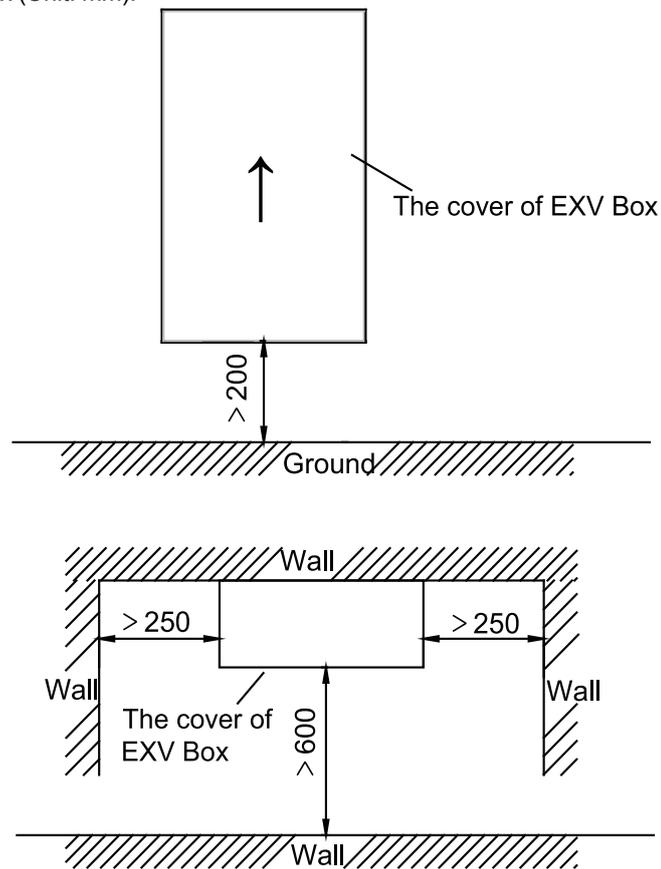
The EXV box must be installed upwards as the direction of the arrow shown in the figure
