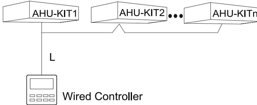
Figure 3-2 One wired controller to several AHU-KITs
