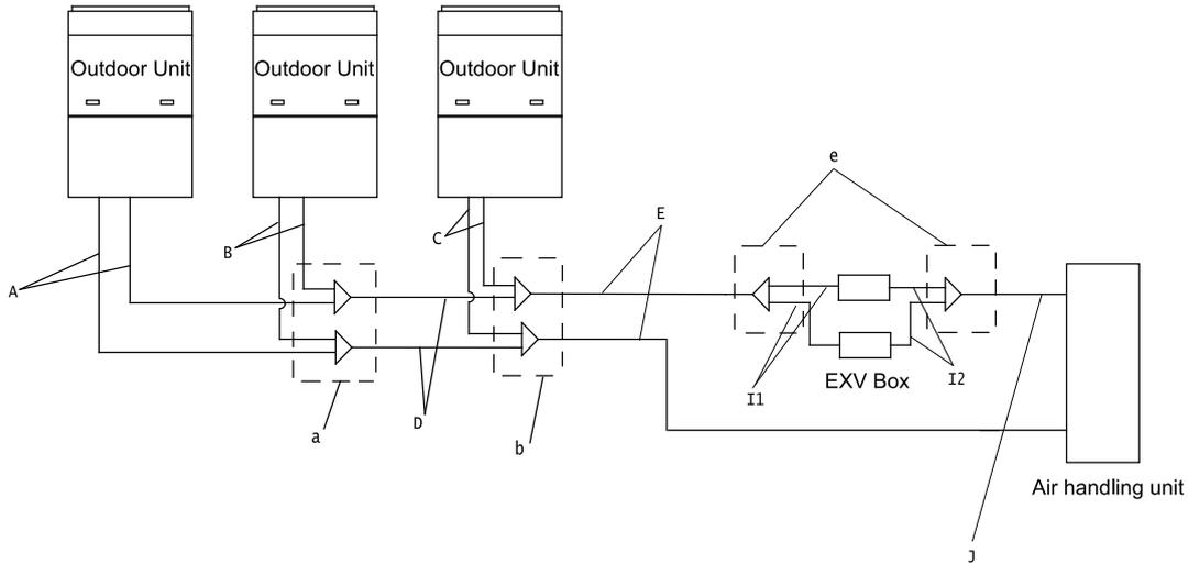
Figure 3-5 Several AHU-KITs to one AHU
