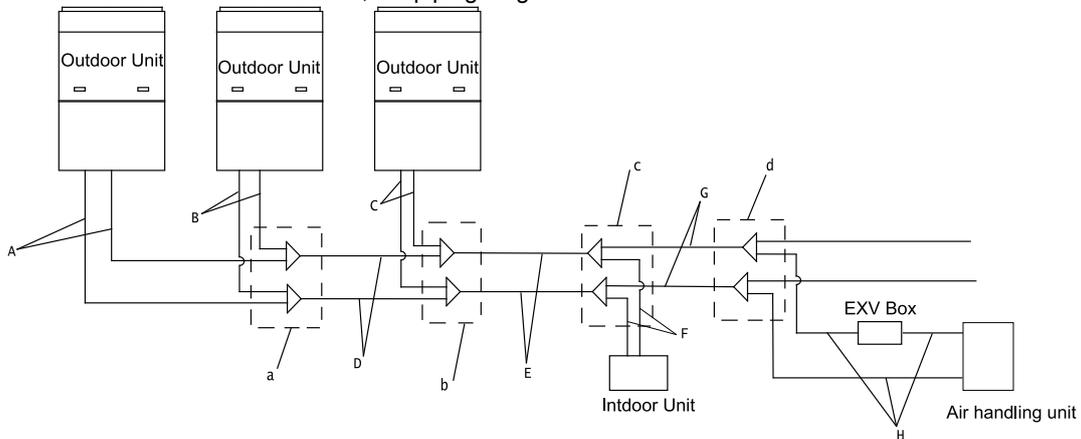
Figure 3-4 One AHU-KIT to one AHU
