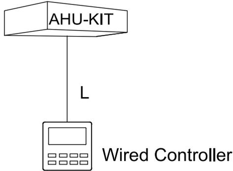
Figure 3-1 One wired controller to one AHU-KIT
