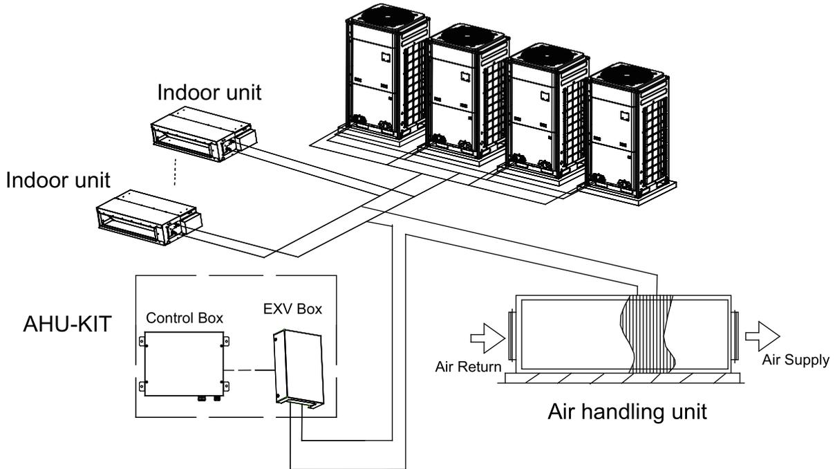
Figure 2-6 AHU-KIT one-to-more (hybrid connection) connection diagram
