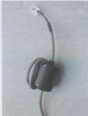
Fig.28 Connection Manner of Crystal Connector, Communication Line and Magnetic Ring
