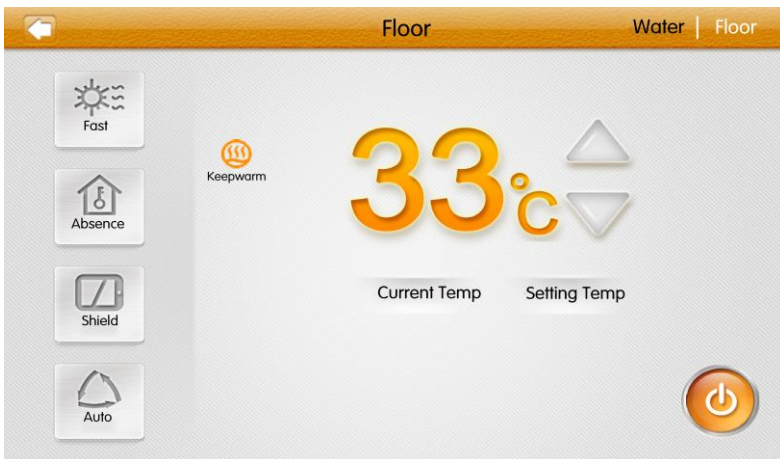
Fig. 3.4 Page of Floor Heating Control
