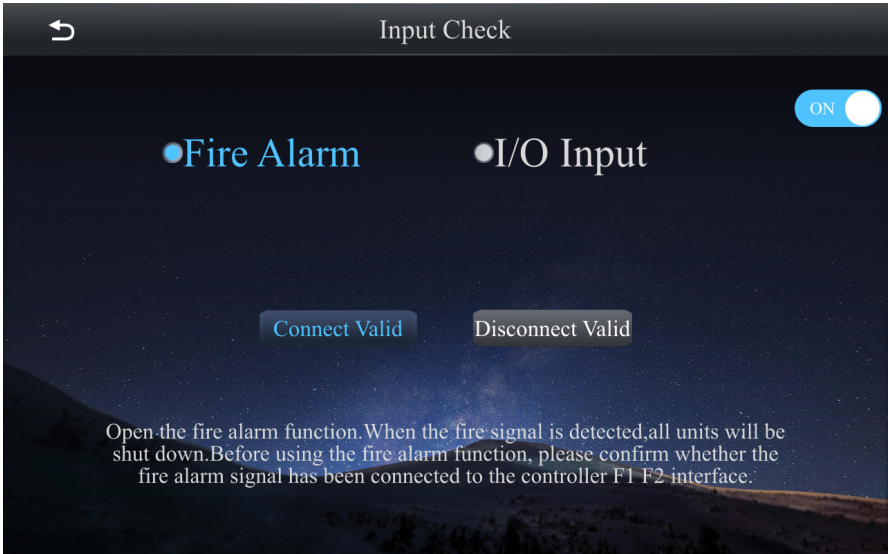
Fig. 5.15 Fire alarm page
