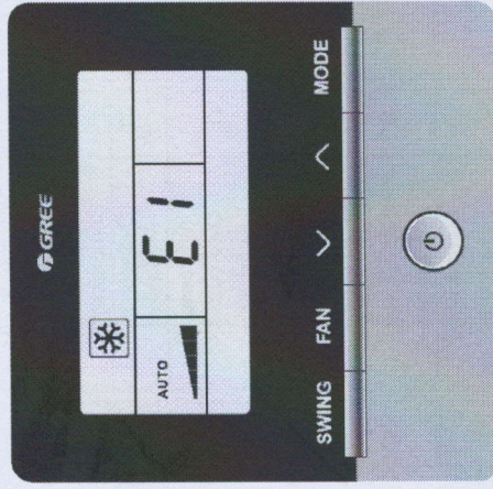
Fig.6.1 Display of outdoor high pressure protection error code
