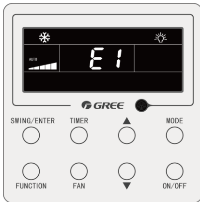
Fig.5.1 Display of Outdoor Unit High Pressure Protection
