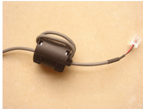
Fig.6.2.5.3 Connection Location of Crystal Connector, Communication Line and Magnetic Ring
