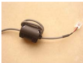
Fig.6.2.6.3 Connection Location of Crystal Connector, Communication Line and Magnetic Ring
