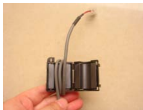
Fig.6.2.6.2 Connection Manner of Crystal Connector, Communication Line and Magnetic Ring
