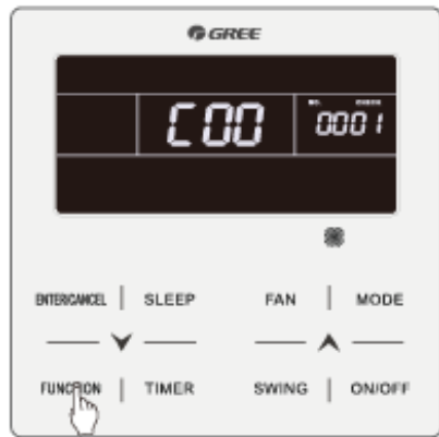
Long press FUNCTION for five seconds when the conditioner is on or off to view parameters.
