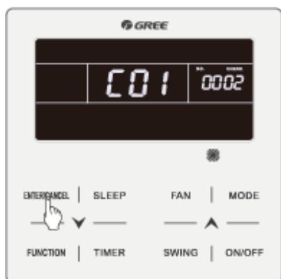
Press ENTER/CANCEL (Note 2) to quit the interface of the indoor unit's engineering number and failure and return to the previous interface.
