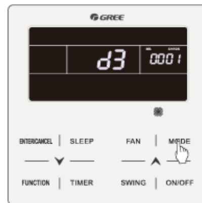
Press MODE to view indoor units' engineering numbers and failures. The engineering number is shown in the timer area, while the failure code is shown in the temperature area (Note 1). Meanwhile, the corresponding failing indoor unit's buzzer buzzes.
