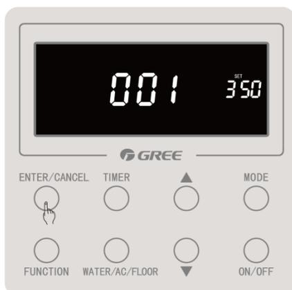
Step 10: Press “ENTER/CANCEL” button to confirm the water tank capacity setting of current hydro box;
