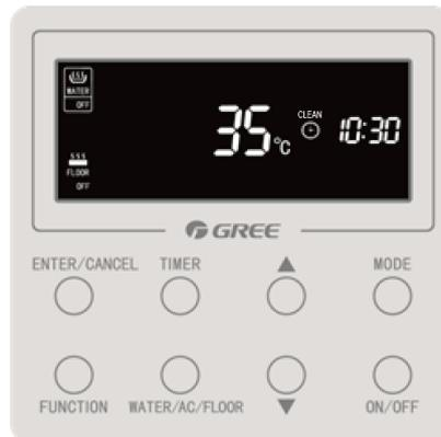
(5) After running for 15~20 minutes, observe the air outlet valve that connects with hydro box during exit pipe engineering construction. When water is flowing out steadily with no air flow, it means evacuation is completed. Then you can close the manual air outlet valve A and stop the hydro box. The operation method is: Press and hold "WATER/AC/FLOOR" for 5s and hydro box will stop cleaning. "Clean" goes off.
