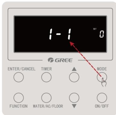
Step 8: Press "MODE" button to enter shunt valve selection setting;
