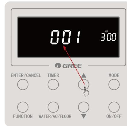
Step 7: Press “▲” or “▼” button to select the sequence(1~3) of hydro box for setting;
