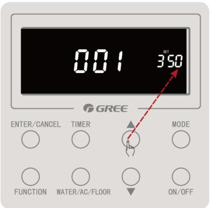
Step 9: Press “▲” or “▼” button to set water tank capacity;
