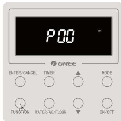
Step 4: Hold on pressing "FUNCTION" button for 5s and then P00 will be displayed;
