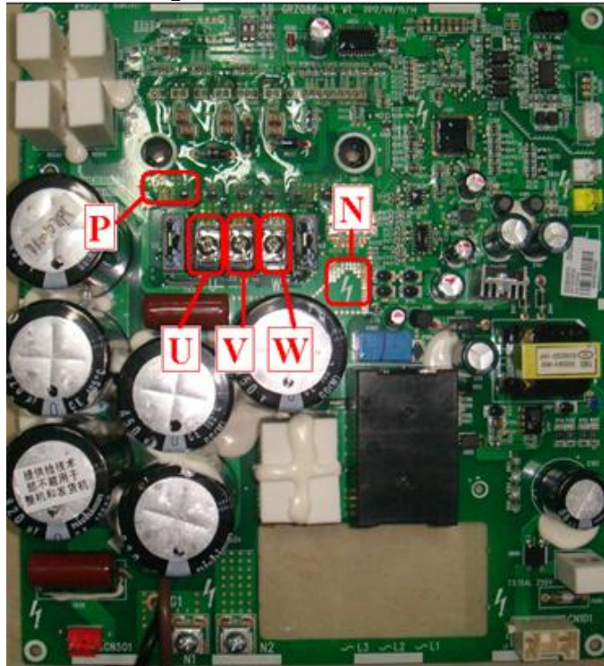
Inverter compressor drive board IPM module over-temperature fault (ODU fault code P8)
