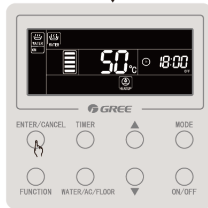
Press the "ENTER/CANCEL" button to cancel power-on timer for water heating
