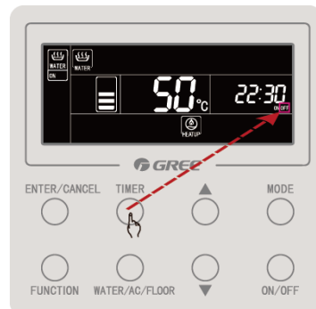
Press the "TIMER" button for twice to switch to power-off timer
