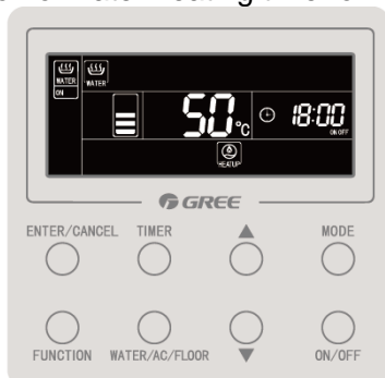
Effective status of water heating timer
