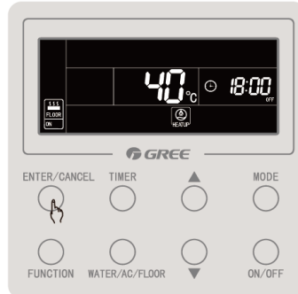
Press the "ENTER/CANCEL" button to cancel power-on timer of floor heating
