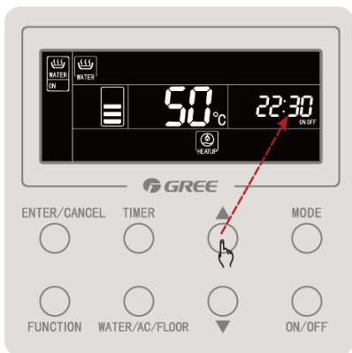
Press the "▲" or "▼" button to set the water heating power-off time
