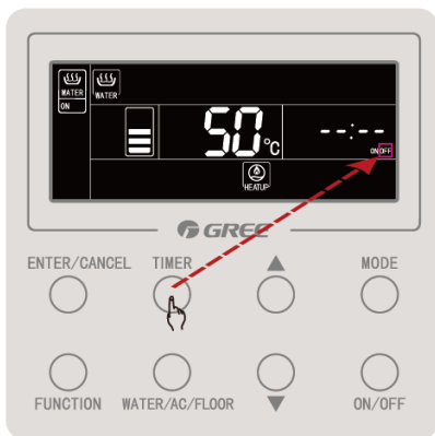
Press the "▲" or "▼" button to set the water heating
