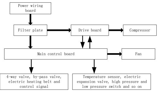
(Bold line is the power line and the slim line is the control line)
