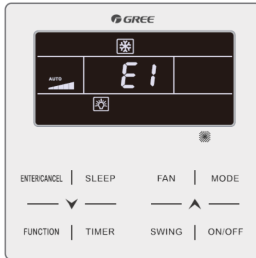
Power-on High-pressure Protection Fault Interface
