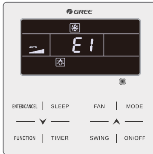
Power-on High-pressure Protection Fault Interface
