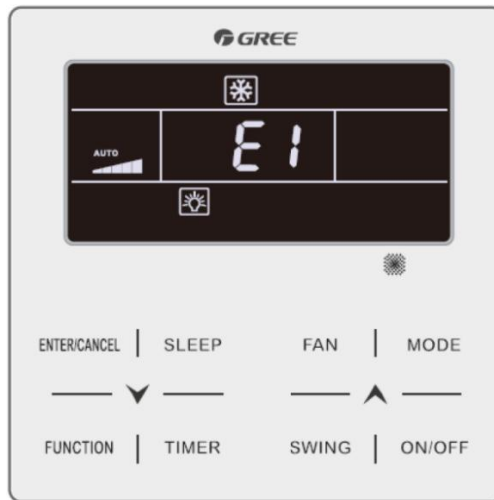
Power-on High-pressure Protection Fault Interface
