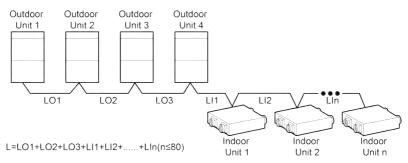
Figure 3-3 Diagram of IDU and ODU control connection
