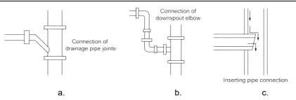
9) Keep the drain pipe downward with an inclination of  $1^{\circ} \sim 2^{\circ}$  or more. Therefore, install a supporter every 1000-1500mm.
