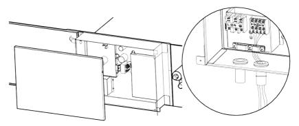
Figure 3-4 Diagram of electric box wiring
