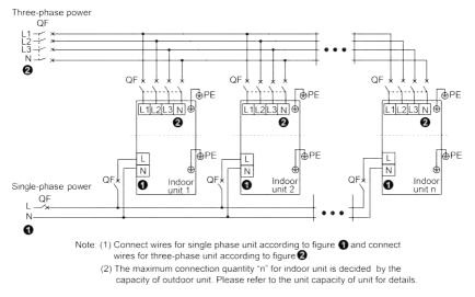
Figure 3-1 Diagram for system electric wiring
