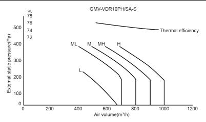
Figure 3-13 The flow/pressure diagram
