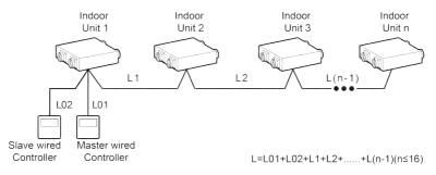
Figure 3-2 Diagram of wired controller control connection
