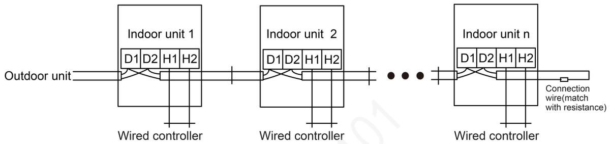
Note: Indoor unit quantity n is according to the outdoor unit capacity.
