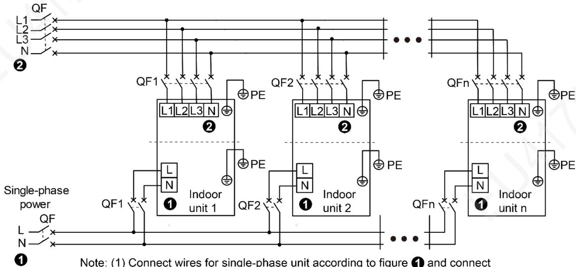
Note: (1) Connect wires for single-phase unit according to figure ① and connect wires for three-phase unit according to figure ②. As for some areas where there's no neutral wire, please refer to the wiring diagram of unit for details.
