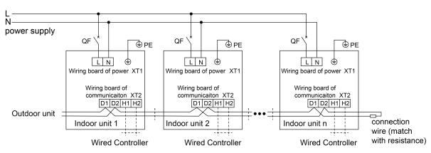
Note: indoor unit quantity n is according to the outdoor unit capacity.
