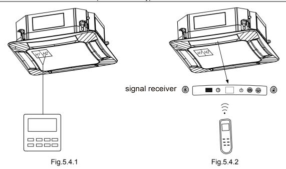
Both IDU and wired controller are equipped with signal receiver, and available for wireless control respectively.
