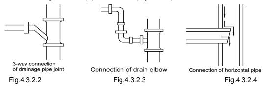
(8) Drainage pipes should have a downward slope of at least 1%~2%, in order to prevent pipes from sagging; install hanger bracket at intervals of 1000~1500mm.
