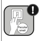
If abnormal condition occurs (e.g. unpleasant smell), please turn off the unit at once and disconnect power supply. Then contact GREE service center. If the air conditioner continues to operate despite of abnormal condition, the unit may be damaged and it may cause electric shock or fire hazard).
