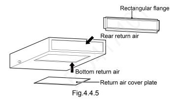
(2) If the bottom return air is desired, just change the place of the rectangular flange and the return air cover plate.
