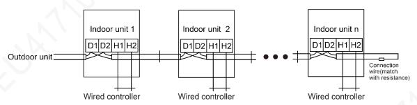
Note:Indoor unit quantity n is according to the outdoor unit capacity.
