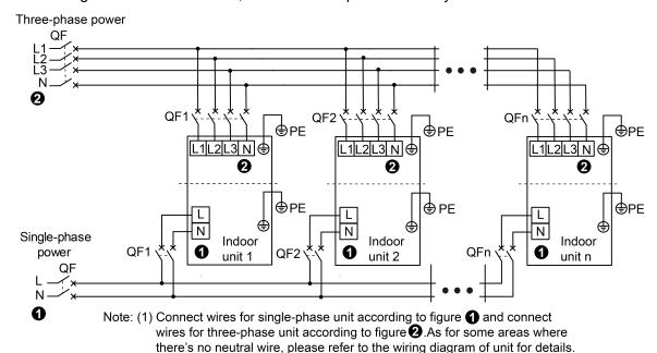
(2) The maximum connection quantity "n" for indoor unit is decided by the capacity of outdoor unit. Please refer to the unit capacity of unit for details.
