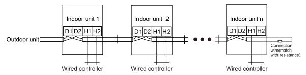
Note:Indoor unit quantity n is according to the outdoor unit capacity.
