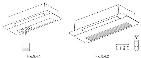
2)Both IDU and wired controller are equipped with signal receiver, and available for wireless control respectively.
