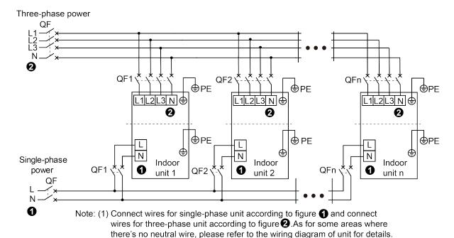
(2) The maximum connection quantity "n" for indoor unit is decided by the capacity of outdoor unit. Please refer to the unit capacity of unit for details.
