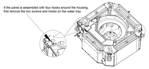
2. Second, remove the 4 screws that secure the indoor unit with water tray;
