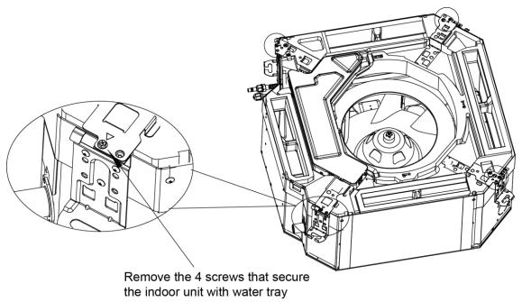
3. Secure the main body with indoor unit by using the screws that are just unscrewed.
