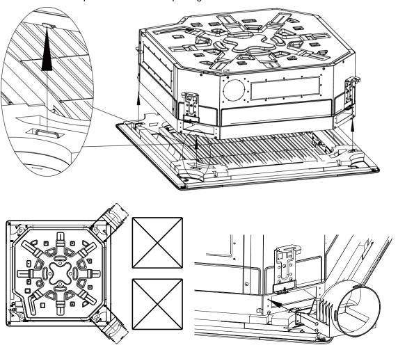
Install the front panel and fresh air opening
