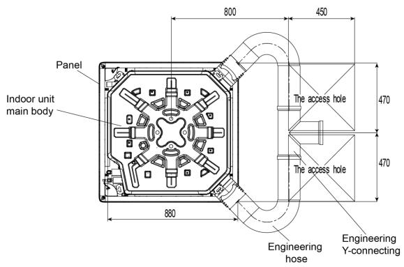
In engineering installation, install the front panel first. Install the fresh air opening from the access hole. Please refer to fig.2 for the dimensions:
