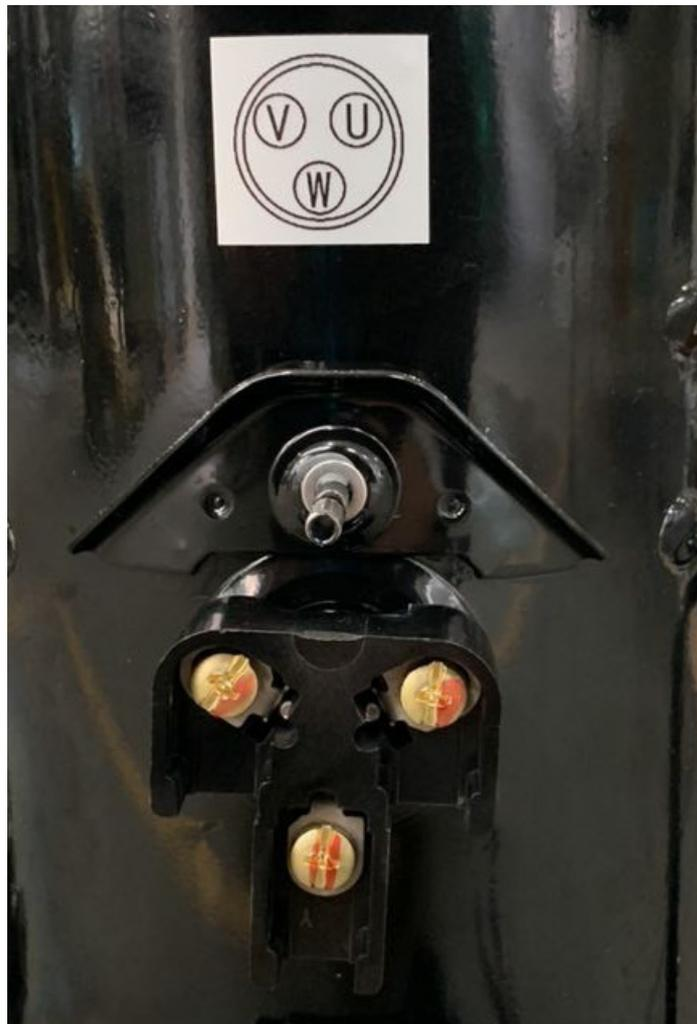
Measure the grounding resistance of each wiring terminal, which should be greater than  $10 \text{ M}\Omega$ ; otherwise, the compressor has an internal fault.
