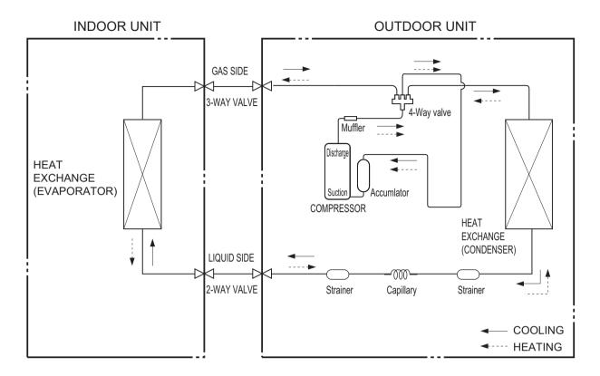
Refrigerant pipe diameter Liquid : 1/4" (6 mm) Gas : 1/2" (12mm)
