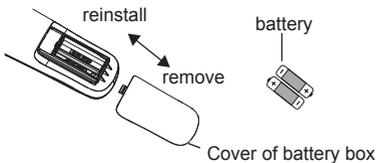
1. Press the back side of remote controller marked with "OPEN", as shown in the fig, and then push out the cover of battery box along the arrow direction.
