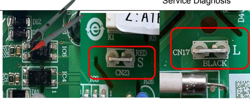
If the voltage is a constant value from DC 0V to DC 5V. Or the voltage between communication line (red) and N (white line) is not close to 18V DC when only indoor charged.
