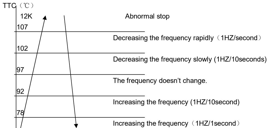
$TTC \geq 107^\circ\text{C}$  lasts for 20 seconds. Overheating protection of air-blowing, alarm malfunction to the indoor, others don't last.
