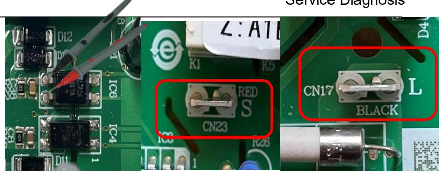
If the voltage is a constant value from DC 0V to DC 5V. Or the voltage between communication line (red) and N (white line) is not close to 18V DC when only indoor charged.
