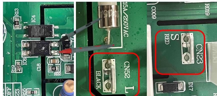
If the voltage is a constant value of 0V DC to 5V DC .Or the voltage between communication line (red) and N (white line) is not close to 18V DC when only indoor charged.
