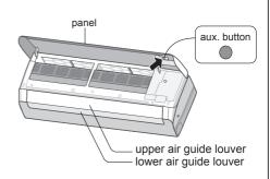
• If remote controller is lost or damaged, please use aux.button to turn on or turn off the air conditioner. The operation in details is as below: As shown in the figure, open panel and press aux.button to turn off the air conditioner. When the air conditioner is turned on, it will operate under auto mode.
