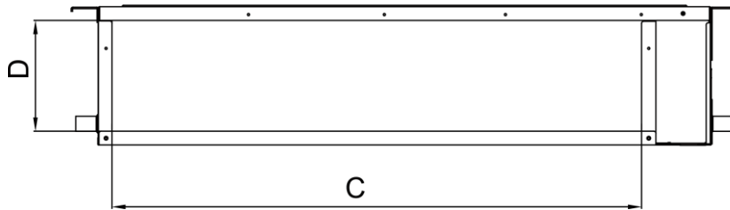
Figure 3-1-20 Return Air Inlet
