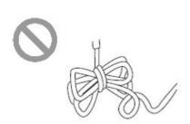
Do not use octopus multipurpose plug or mobile terminal board for wire connection.
