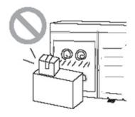
It may reduce efficiency or cause stop of the unit and even fire. Keep pressurized spray, gas holder and so on away from the unit above 1m.
