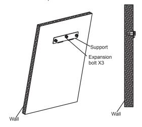
Step3: Attaching indoor unit to the wall.
