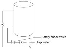
Note: for safe use of water, water outlet/inlet of water tank must connect with a certain length of PPR pipe, L≥70×R2(cm, R is inside radius of the pipe). Moreover, heat preservation should be conducted and metal pipe cannot be used. For the first use, water tank must be full of water before the power is on.
