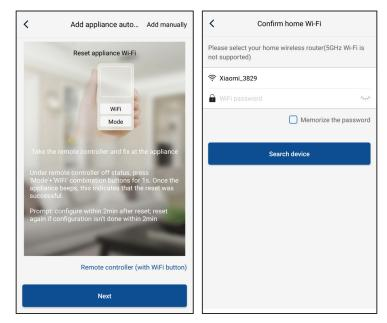
Reset the air conditioner (refer to the operation instructions in APP interface) and click "Next" to add home appliance automatically (Wi-Fi password shall be input). Or after setting and energizing the air conditioner, click "Add appliance manually" at the right upper corner to select the wireless network for controlling the device. Then confirm family Wi-Fi and arrange configuration.
