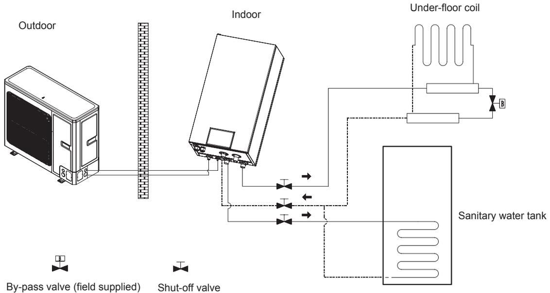
Note: sanitary water tank should be equipped with internal electric heater to secure enough heat energy in the very cold days.
