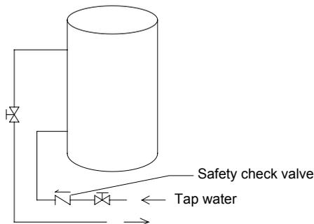
Note: for safe use of water, water outlet/inlet of water tank must connect with a certain length of PPR pipe,  $L \geq 70 \times R2$  (cm, R is inside radius of the pipe). Moreover, heat preservation should be conducted and metal pipe cannot be used. For the first use, water tank must be full of water before the power is on.
