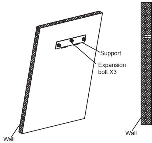
Step3: Attaching indoor unit to the wall.
