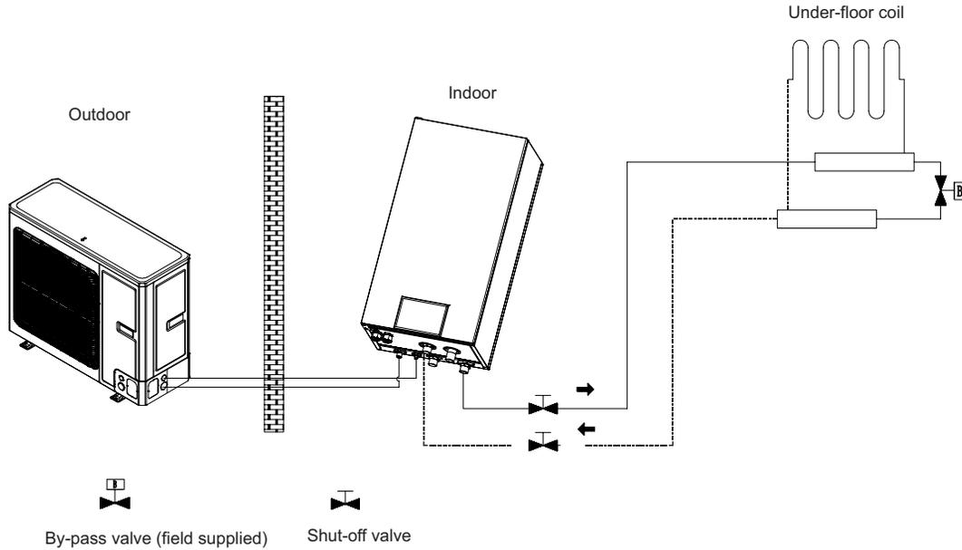
Note: the bypass valve must be installed to secure enough water flow rate, and should be installed at the collector.
