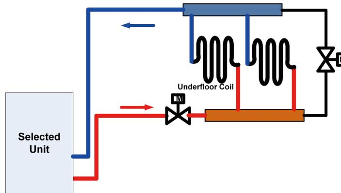
Length of underfloor coils is recommended to be within 100m and length of each branch should be kept the same to the most extent.
