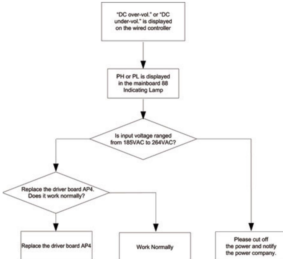
Note: three-phase input voltage is in the range from 320VAC to 475VAC.
