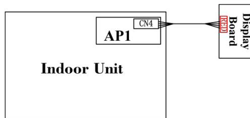
Notes: the wired controller can be connected to the terminal of AP1 CN4 with the four-wire communication cable.
