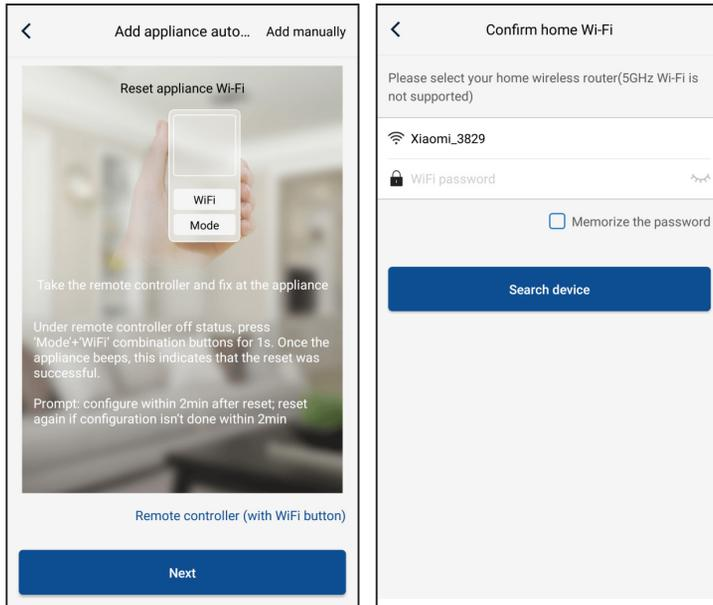
Reset the air conditioner (refer to the operation instructions in APP interface) and click **“Next”** to add home appliance automatically (Wi-Fi password shall be input). Or after setting and energizing the air conditioner, click **“Add appliance manually”** at the right upper corner to select the wireless network for controlling the device. Then confirm family Wi-Fi and arrange configuration.
