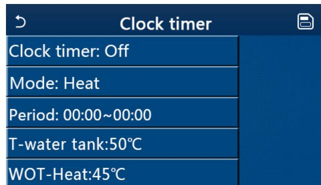
3. The option “**Mode**” is used to time the desired mode; “**WOT-Heat**” and “**T-water tank**” is used to set the corresponding water temperature; “**Period**” is used to for time setting. After that, by touching the “**Save**” icon, all settings will be saved.
