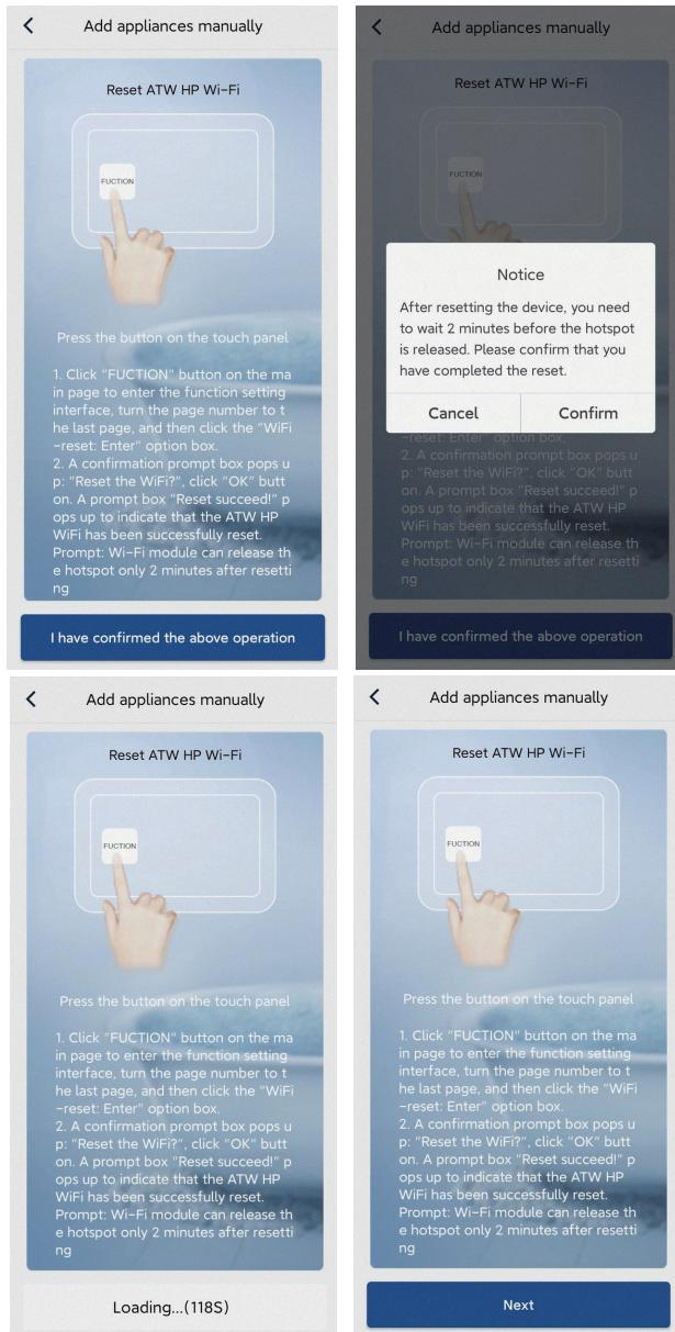
Reset the air conditioner (refer to the operation instructions at APP interfaces), click “OK” and wait for two minutes. Then, click “Next” to select the wireless network for the device to be controlled. After that, confirm the family Wi-Fi and do the configuration.
