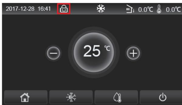
In this case, the control panel is locked and any touch operation does not work. By touching for six seconds, the control panel will be unlocked and touch operation will work. However, the setting of “**Child Lock**” will remain to be “**On**”, and if there is no any operation in 30 seconds, the control panel will be locked again.
