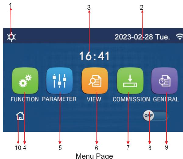
Above the menu, the corresponding icon will be displayed based on the mode and status of the control panel.
