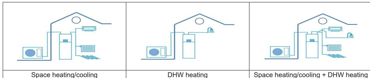
There are five basic working modes, including space cooling, space heating, domestic water heating, space cooling plus domestic water heating, and space heating plus domestic water heating.
