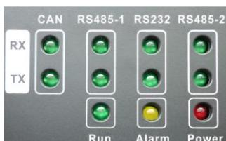
The above LED indicator is mainly consist of two parts: status indicator (run, alarm, power) and communication indicator (CAN, RS485, RS2332). The following table is the working status of each indicator.
