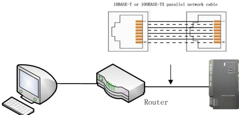
(2) Communication line connection between BACnet gateway and AC units:
