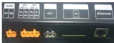
**CAN communication interface:** connect it to the AC unit through the 2-core communication line to realize the communication between BACnet gateway and the AC which adopts CAN protocol.
