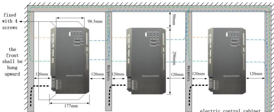
**⚠ Warning!** Power cord and communication line of BACnet gateway must conduct routing separately(the distance shall be over 15cm); otherwise, it might lead to BACnet gateway communication malfunction!
