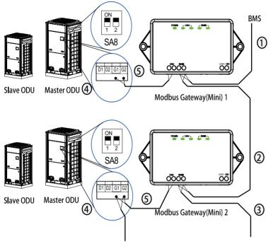
(1) Communication wire connection between Modbus Gateway(Mini) and BMS: Step 1: Confirm the first Modbus Gateway(Mini) (Modbus Gateway(Mini)1 as shown in the figure) that needs to be connected to BMS. Connect the port of RS485 of this gateway and the BMS with communication cable, as shown in step ① in the figure.
