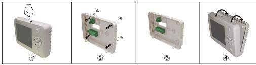
Step 1: Press the button at the top of the wired controller to remove the front panel and the bottom plate.
