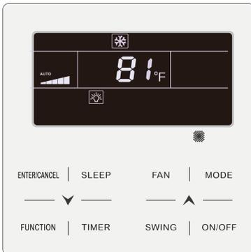
Fig. 6.3 Interface of On status in Fahrenheit
